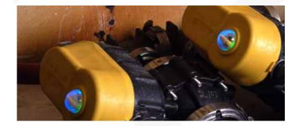
LED provides valve performance feedback indicating blue for power and yellow for a fuse blown condition. With the optional open / close verify, the LED indicates green and red, respectively. As an additional option, EVX reports temperature, voltage and cycle count.
