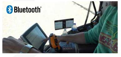
EVX offers the latest communication protocol options including CAN/ ISO BUS, Pulse-Width-Modulation (PWM), and Bluetooth®\* wireless technology. Diagnostic options report voltage, temperature, and cycle count to warn of concerns before they become problems.
