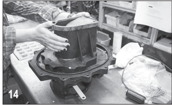
14 Install check valve onto diffuser.
