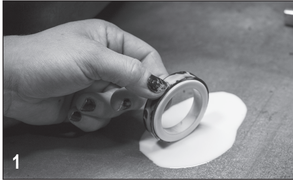
1 Clean the new seals thoroughly and lubricate with P80 lubricant.
