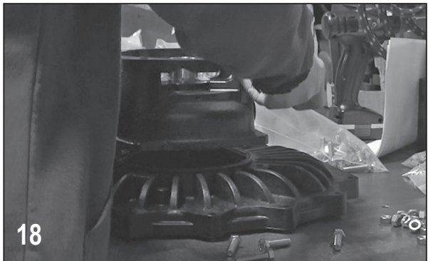
Remove the reservoir assembly from the rear bracket. The rotating half of the seal can now be removed from the shaft.
