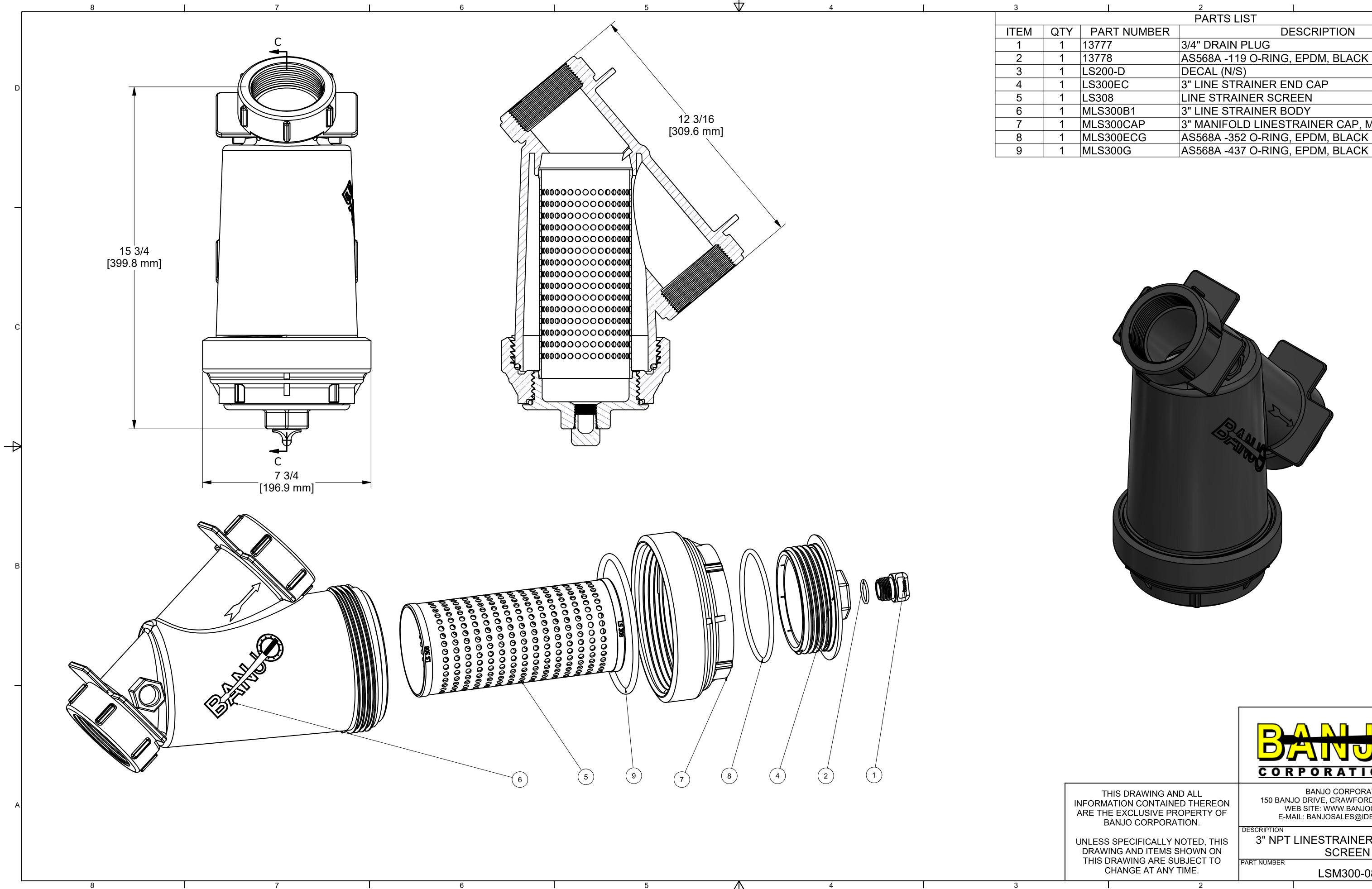
DESCRIPTION AS568A -119 O-RING, EPDM, BLACK 3" LINE STRAINER END CAP 3" MANIFOLD LINESTRAINER CAP, MACHINED AS568A -352 O-RING, EPDM, BLACK
