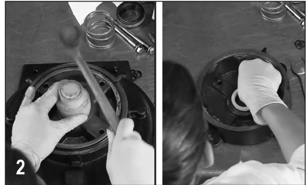
2 Install the ceramic seal into the rear bracket and reservoir. . A flat uniform object and rubber mallet can be used to install the ceramic seal. Use caution when applying pressure as the ceramic seals are fragile and may crack.
