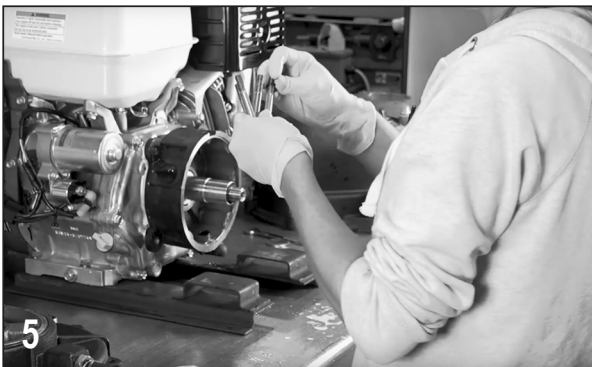
5 Clean the rear bracket bolts, making sure they are free from damage. Replace the rear bracket bolt o-rings with new.
