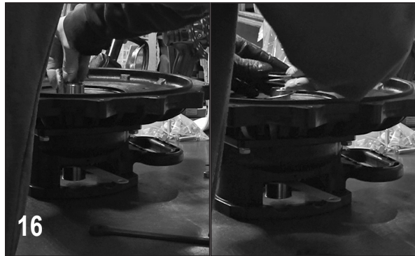
16 Remove the seal spring and retainer.
