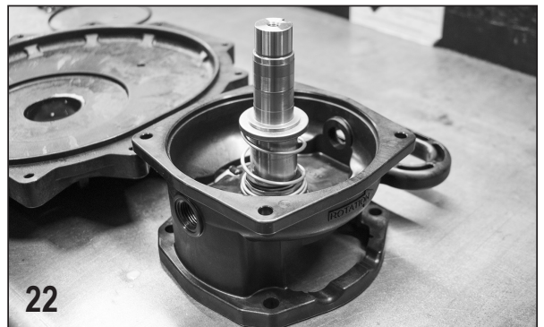
22 Remove seal and shaft from reservoir and separate seal from shaft.
