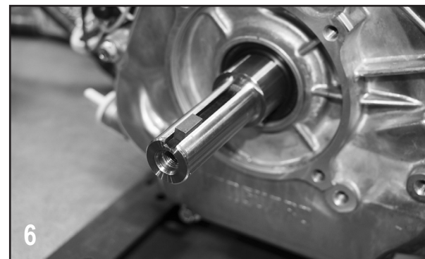
Remove the key from the shaft.
