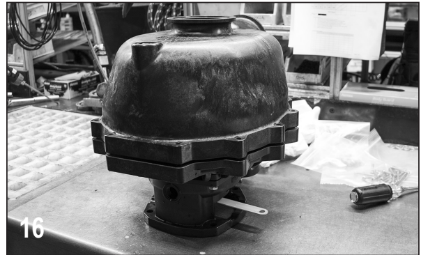
16 Place body onto the rear bracket assembly ensuring the check valve groove is aligned correctly. If pump body is fully seated, body bolts will drop into place without resistance.
