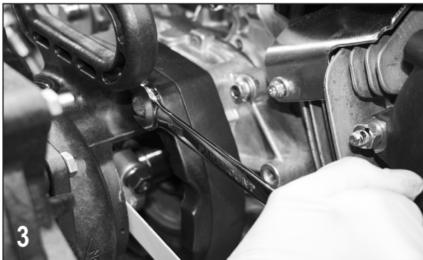
Remove bolts and lock washers on the back of the wet seal reservoir.
