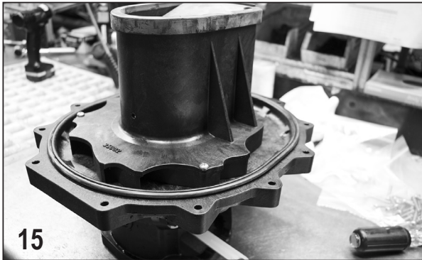
15 Place the body O-ring into the groove on the rear bracket.
