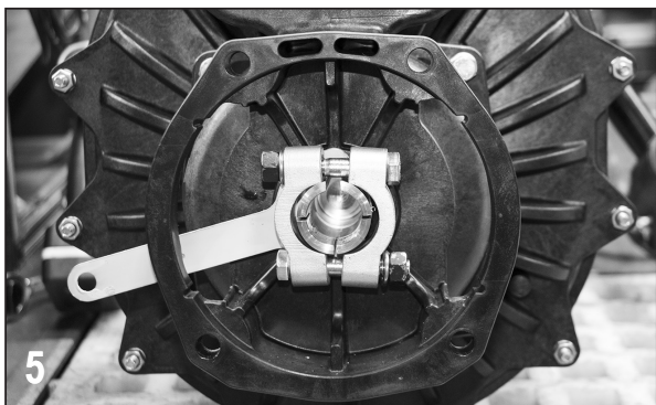
Remove the clamp from the shaft.
