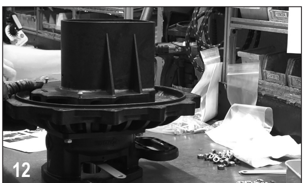
Remove screws and diffuser.
