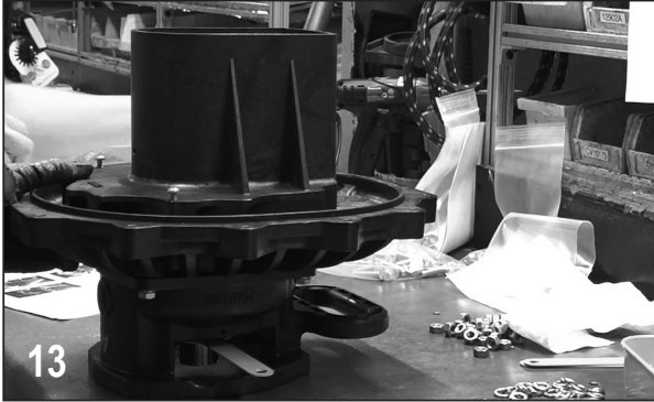
13 Install diffuser and tighten screws to 20-40 in-lb.
