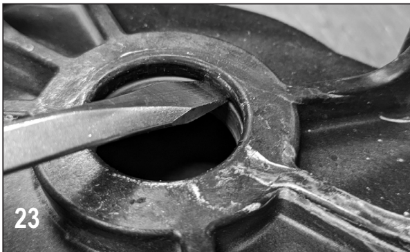
Remove the 2 ceramic seals from the reservoir and rear bracket. A wide flat bladed screwdriver may be used to carefully pry the seals out. Use caution when applying pressure as the ceramic seals are fragile and may crack. Set aside the seals.
