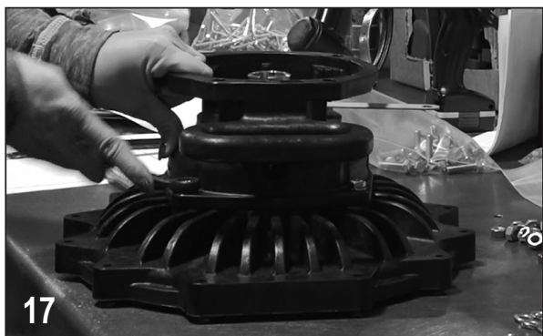
17 Remove bolts from the back of the reservoir.
