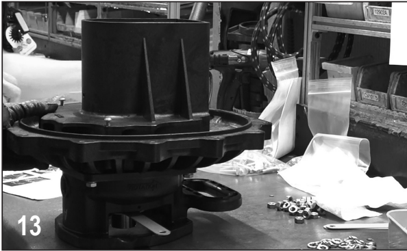
13 Install diffuser and tighten screws to 20-40 in-lb.
