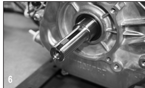
6 Remove the key from the shaft.
