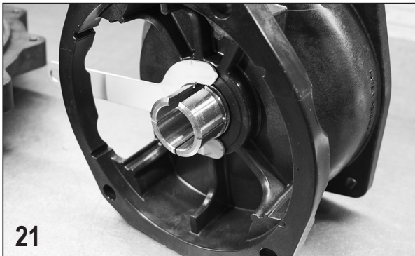
Remove the yellow spacer on back side of reservoir.
