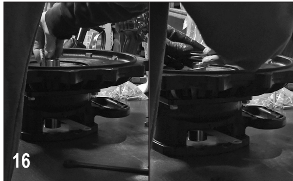
16 Remove the seal spring and retainer.
