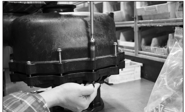
Remove body bolts, lock washers, and nuts.
