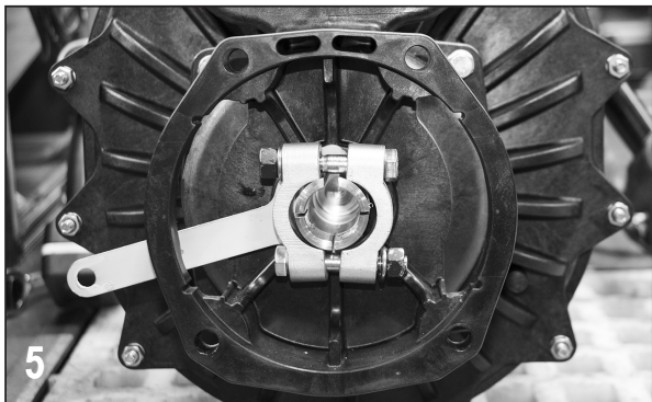
5 Remove the clamp from the shaft.
