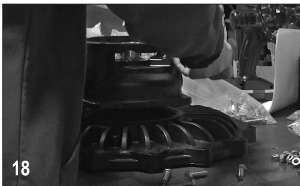
18 Remove the reservoir assembly from the rear bracket. The rotating half of the seal can now be removed from the shaft.
