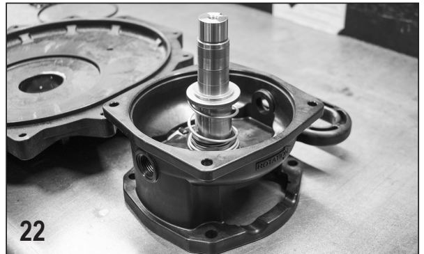
Remove seal and shaft from reservoir and separate seal from shaft.
