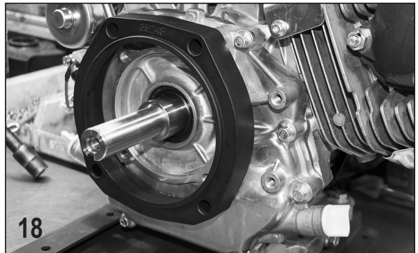
18 Place spacer on the engine for gas models.
