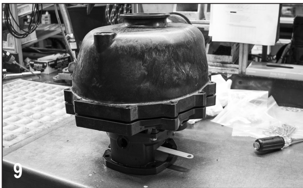
Remove body from the rear bracket assembly.
