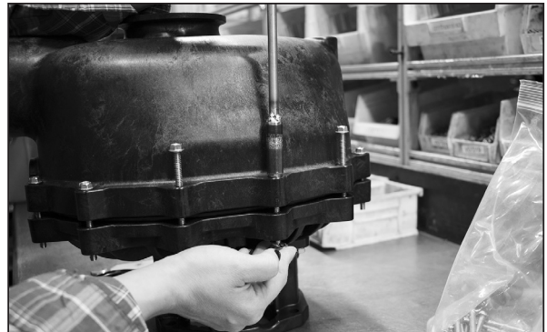
Remove body bolts, lock washers, and nuts.
