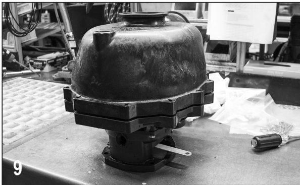
Remove body from the rear bracket assembly.
