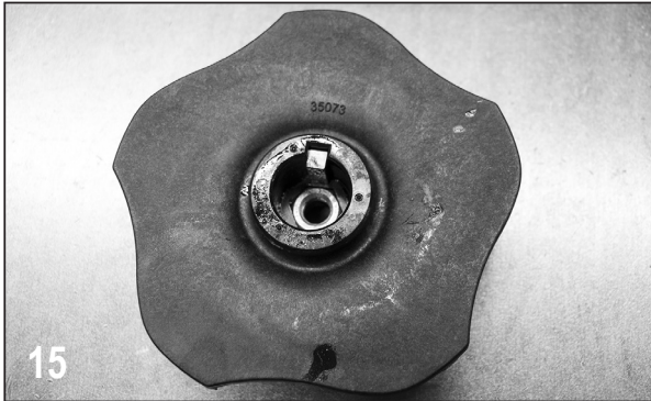
15 Remove hex nut and key from the impeller.
