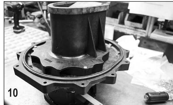
Remove the body O-ring from the groove on the rear bracket.
