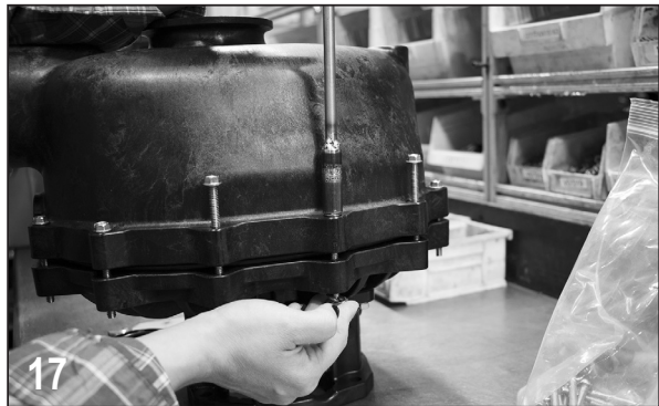
17 Insert and tighten body bolts, lock washers, and nuts to 75-100 in-lb.
