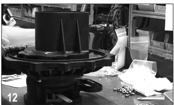
Remove screws and diffuser.
