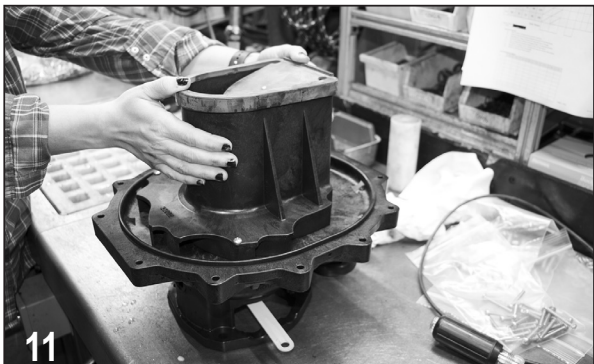
Remove check valve from diffuser.
