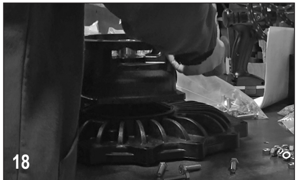
18 Remove the reservoir assembly from the rear bracket. The rotating half of the seal can now be removed from the shaft.
