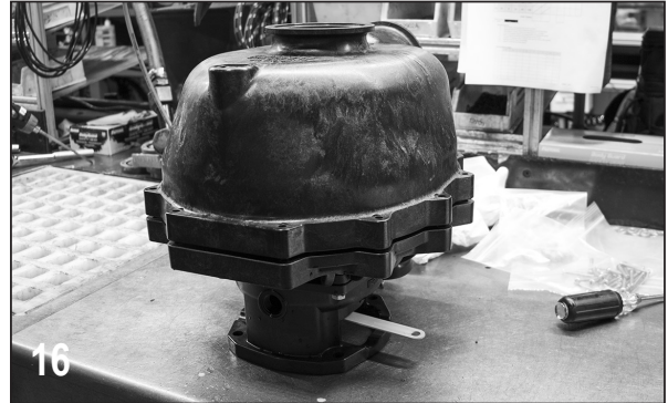
Place body onto the rear bracket assembly ensuring the check valve groove is aligned correctly. If pump body is fully seated, body bolts will drop into place without resistance.
