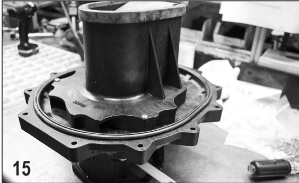
Place the body O-ring into the groove on the rear bracket.
