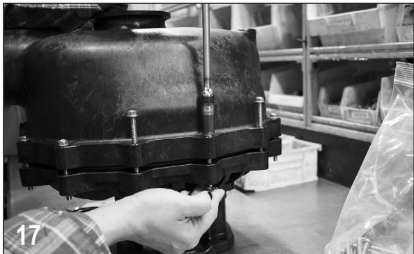
Insert and tighten body bolts, lock washers, and nuts to 75-100 in-lb.
