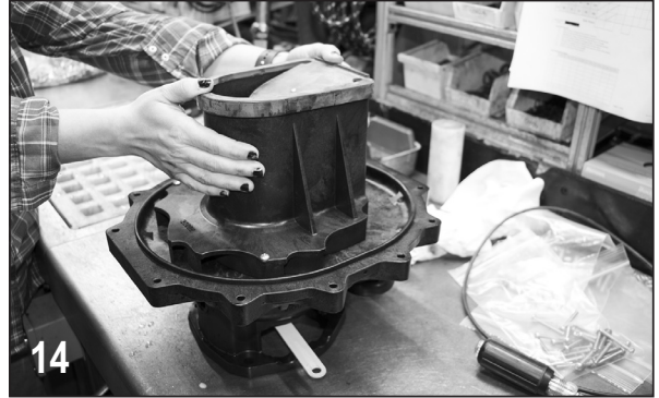
Install check valve onto diffuser.
