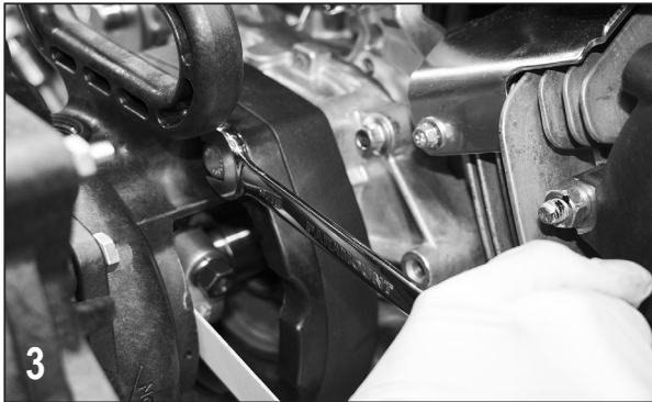
3 Remove bolts and lock washers on the back of the wet seal reservoir.
