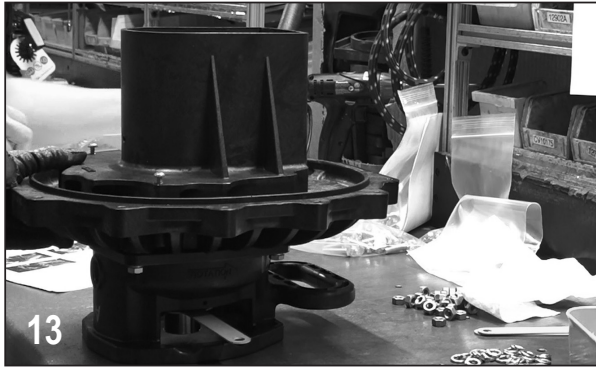
13 Install diffuser and tighten screws to 20-40 in-lb.
