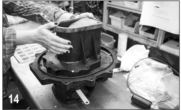
14 Install check valve onto diffuser.
