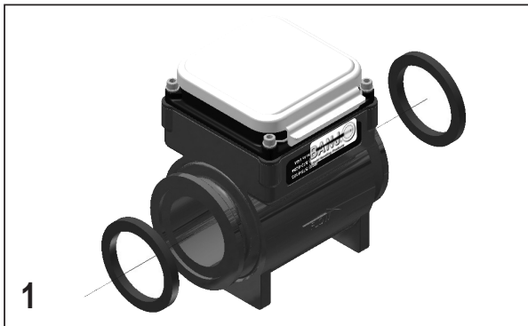
1 Position gasket at either end. Note: if hose is used, smooth bore is recommended.
